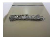
Failure in tensile test
