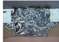
Failure in tensile test
